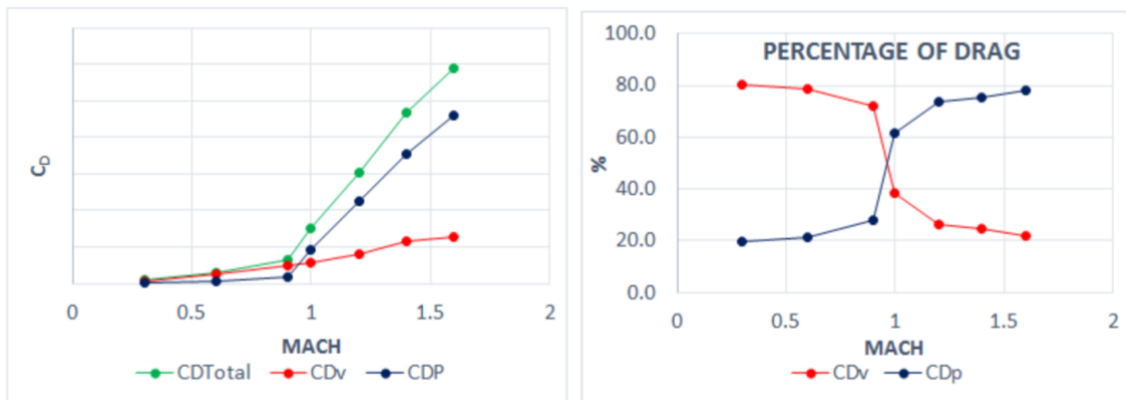
Figure 13: Variation of drag coefficients of the F16 fighter jet with Mach number
