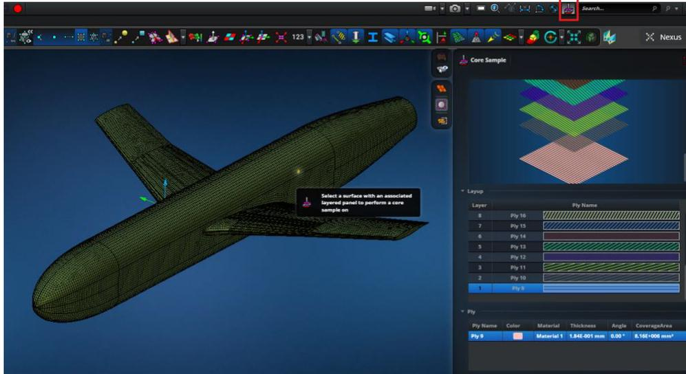
Figure 8: "Core Sample" Tool in MSC Apex Interface
