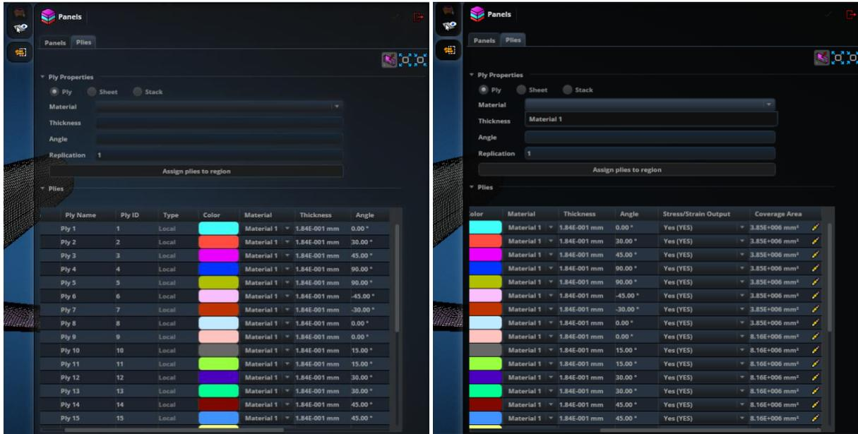
Figure 6: Display of Plies in the “Panel” Tab in the MSC Apex Interface
