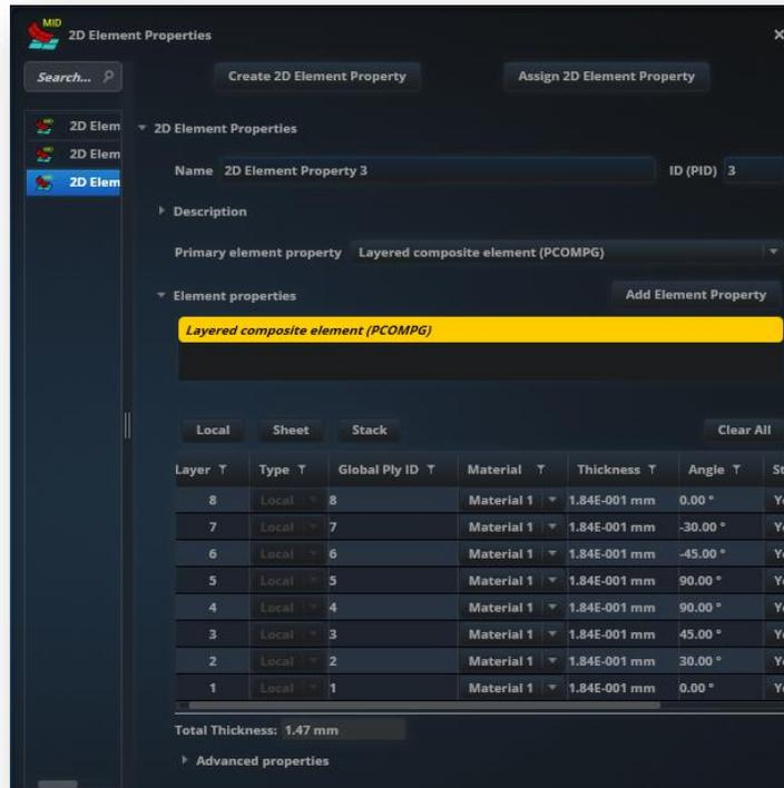
Figure 4: “2D Element Properties” Tab in MSC Apex Interface
