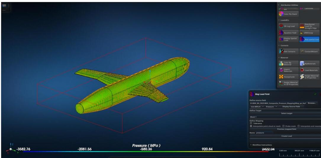
Figure 11: Preview of the Region to be Mapped in the “Map Load Field” Tool in MSC Apex Interface
