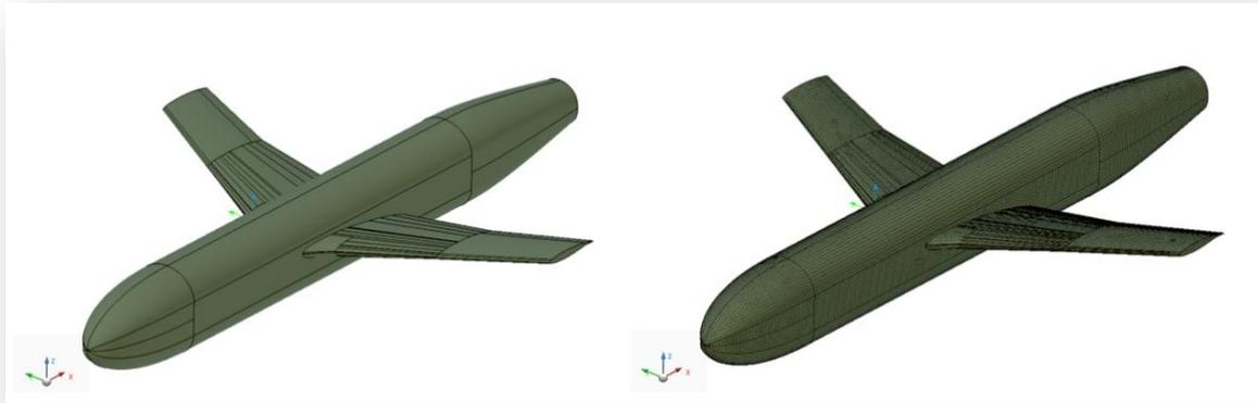
Figure 2: NASA Wing-Fuselage Junction Surface and Finite Element Model
