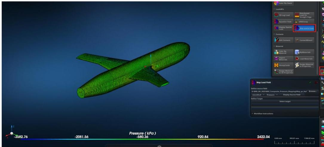
Figure 10: “Map Load Field” Tool in MSC Apex Interface
