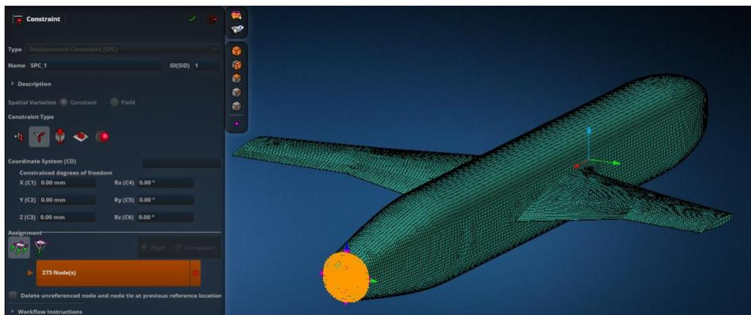
Figure 9: Boundary Conditions of Wing-Fuselage Connection Model
