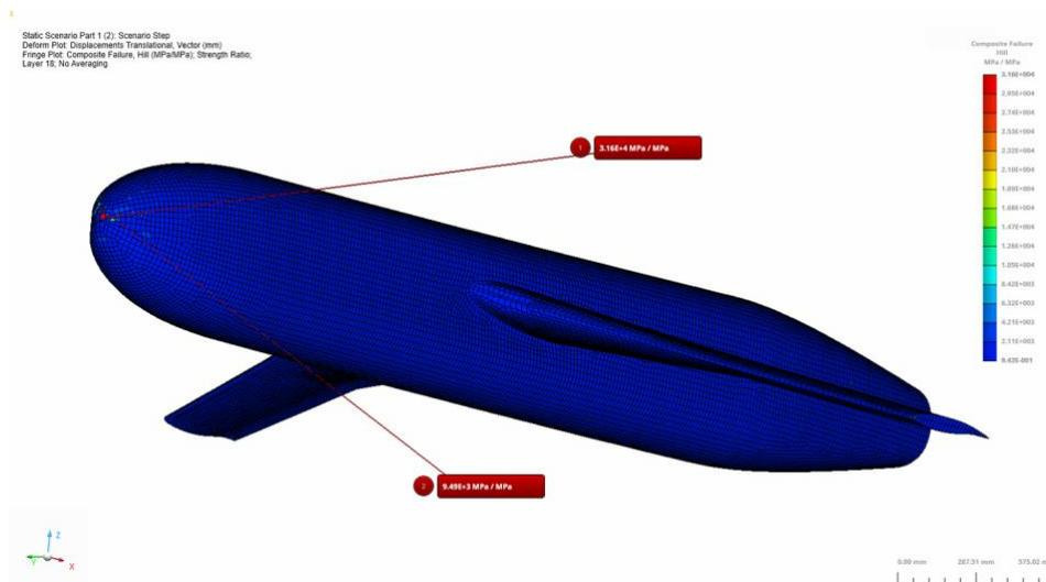
Figure 13: Strength Ratio (Hill) Results for a Sample Layer (18 Layer) in the Wing-Fuselage Connection Model
