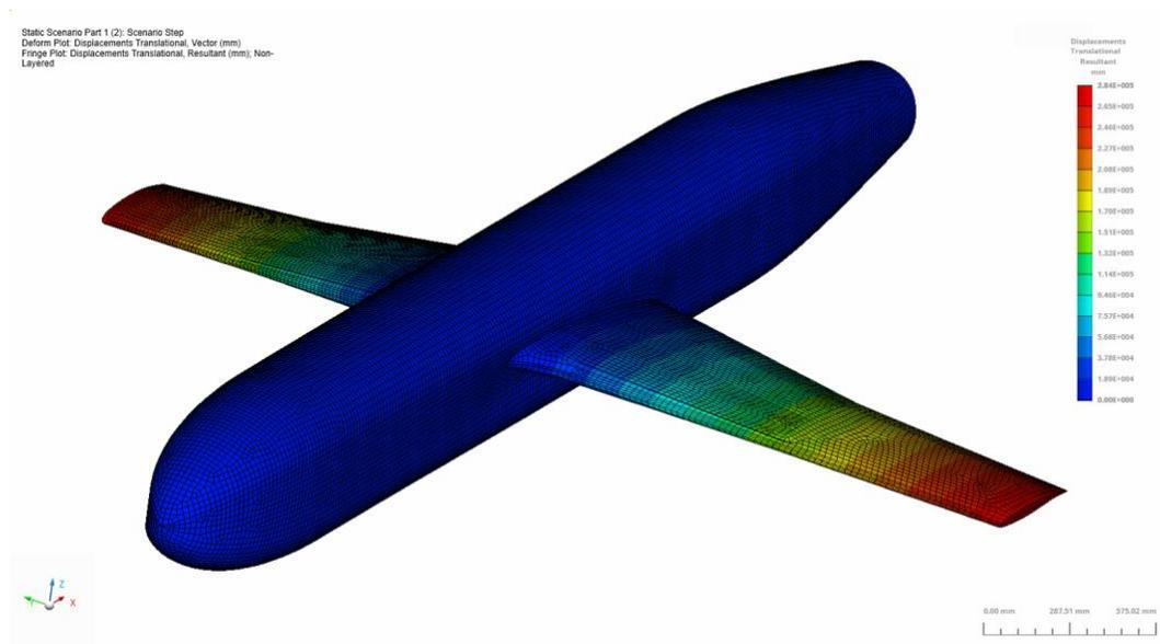
Figure 14: Translational Displacement Results of Wing-Fuselage Connection Model
