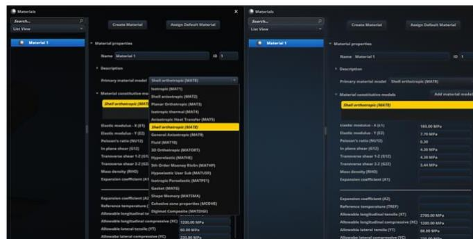
Figure 3: Orthotropic Material Model and Mechanical Properties in MSC Apex Interface
