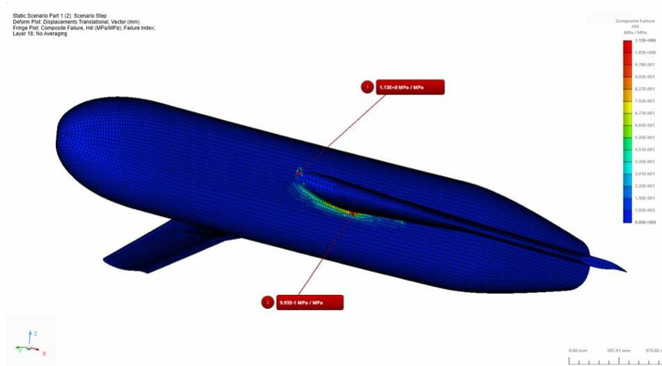
Figure 12: Failure Index (Hill) Results for a Sample Layer (18 Layer) in the Wing-Fuselage Connection Model
