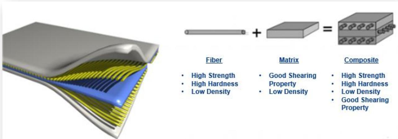
Figure 1: Composite Material Content
