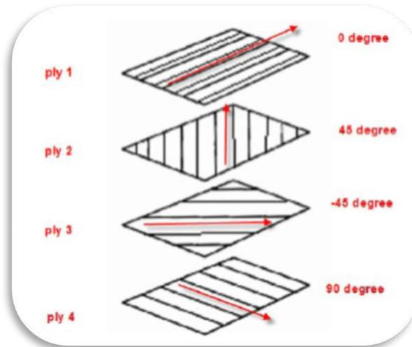
Figure 5: Laminar Model Consisting of Four Ply
