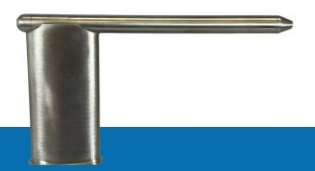
Pitot-Static Probes measure total and static pressures to derive airspeed and altitude. Commonly used for flight applications, these probes can be straight for boom mounting ahead of the aircraft or include an aerodynamic strut for fuselage mounting.
