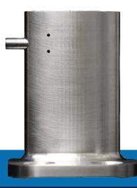
Our flight specific TAT Probes are designed to reduce errors associated with radiative heat transfer, withstand varied environmental conditions, and operate at velocities up to Mach 1. TAT Probes can be manufactured in a variety of configurations for use in flight, engine and wind tunnel testing, and even integrated with other air data solutions.
