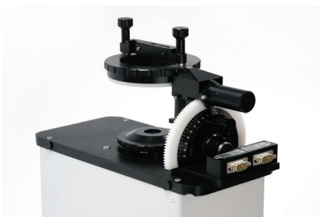
Manual and motorized pitch-yaw manipulators allow probe rotation around two axes during directional calibration.
