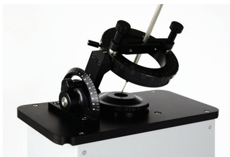
Manual and motorized pitch-yaw manipulators allow probe rotation around two axes during directional calibration.
