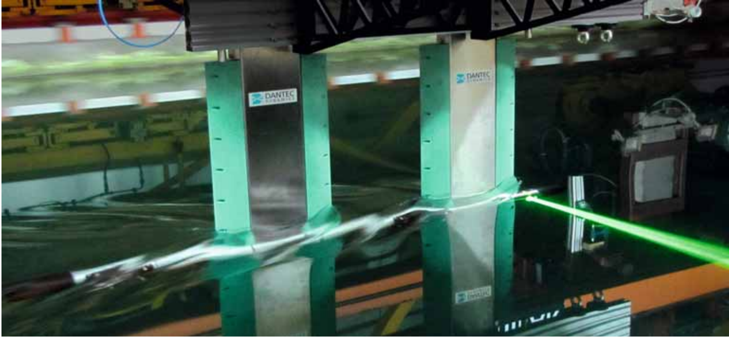
Customized Stereoscopic underwater PIV systems for towing tanks. Courtesy of CEHPAR, Spain
