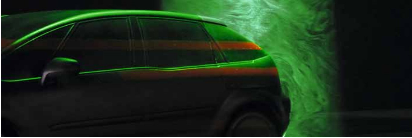
Time-Resolved PIV measurement of wake flow behind a car. Courtesy of PSA, France
