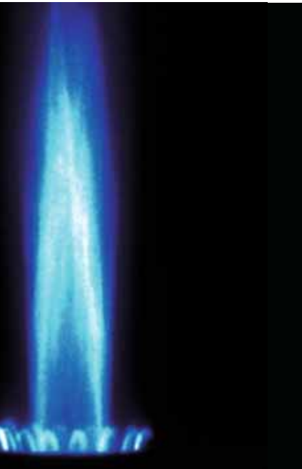
OH* chemiluminescence from a slightly turbulent atmospheric flame at around 308 nm with exposure times of 100 \mu s, 1 ms and 10 ms respectively.
