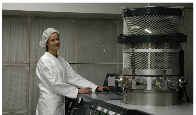
Thin film coating in Dantec Dynamics' clean room facility.
