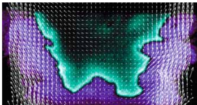
Simultaneous flow field, fuel mauve and OH green visualisation in a turbulent atmospheric flame. Courtesy of R. Collin and P. Petersson, Division of Combustion Physics, Lund University, Sweden.
