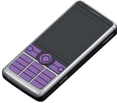
Model for Drop Test Simulation By courtesy of Sony Ericsson Mobile Communications AB
